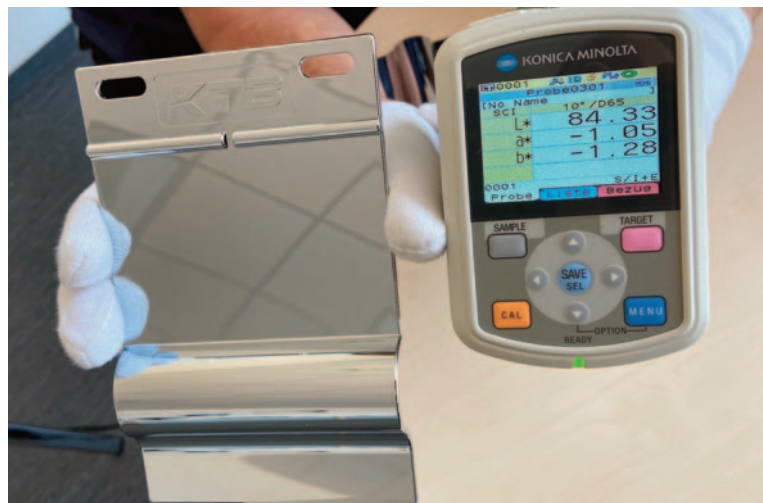
Colour measurement with Konica Minolta CM-700d
